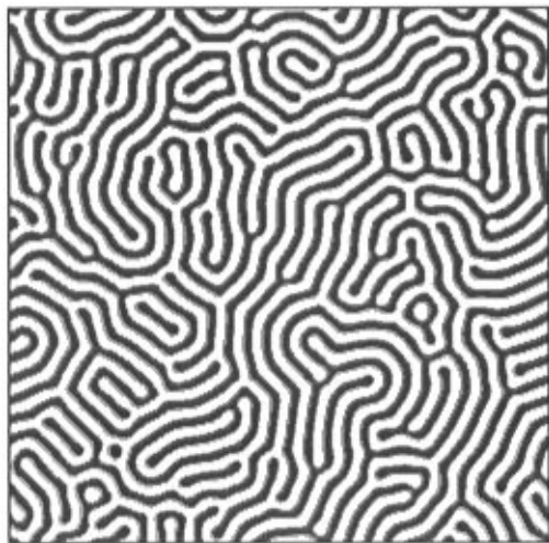
Figure 2. Density profile of the randomly oriented lamellar structure obtained by the simulation with \dot{\gamma} = 0 iterated for 10^5 steps.
